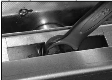
Figure 7 – Tighten the shaft bolt using wrench # 24
