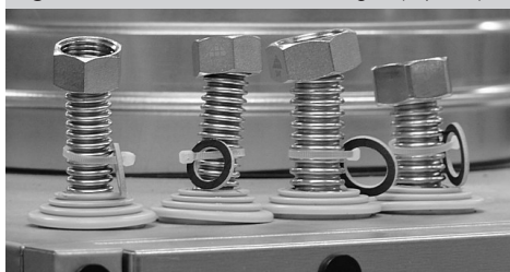
Figure 11 – Connection of heat-exchangers (cap nuts)
