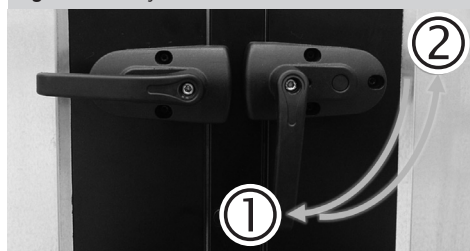
Figure 4 – Safety door lock
