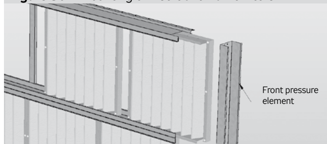
Figure 30 – Mounting of insert and frame filters
