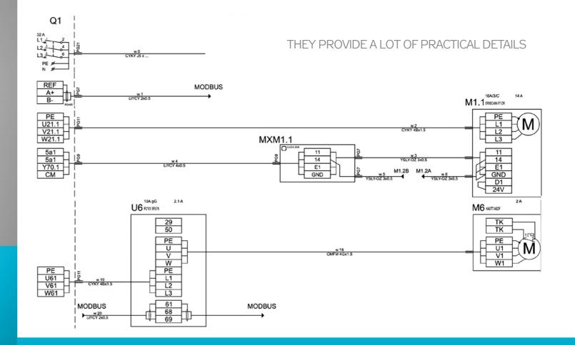
Along with the VCS control unit we provide the complete control project i.e. wiring schemes, specification of the wire sizes, connectors assignment, drives (VFD), controllers and sensors. So there is no need to do specific and expensive control designing. The delivered components are factory preset, the unit can be put into operation by a briefed electrician.
