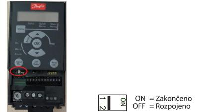
• For the Danfos Basic frequency inverter, the terminal resistor is set using a switch.
