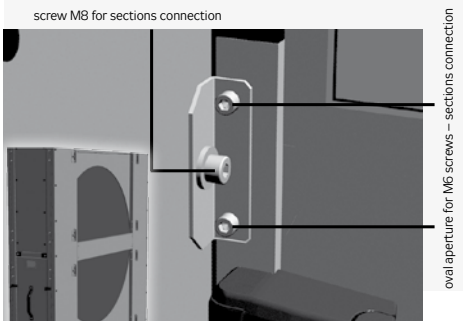
Fig. 13 – connection by means M8 screws and rectangular couplings
