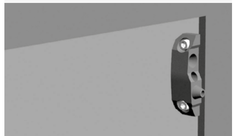
Fig. 12 – sections connection (connectors + M8 screw)
