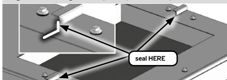
Fig. 26 – sealing of roof parts (PU sealant) -F
