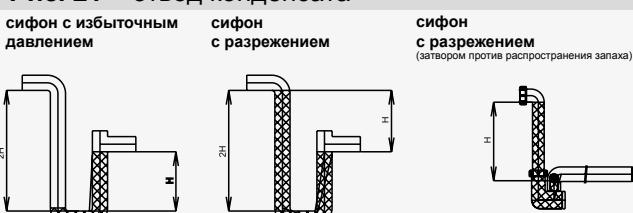
$$H_{min} (\text{mm}) = P (\text{Pa}) / 10$$
