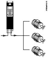
VLT 6000 HVAC is able to control several motors connected in parallel. If the motors are to have different rpm values, the motors must have different rated rpm values. Motor rpm is changed simultaneously, which means that the ratio between the rated rpm values is maintained across the range. The total current consumption of the motors is not to exceed the maximum rated output current  $I_{VLT,N}$  for the frequency converter.
