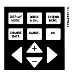
DISPLAY MODE [DISPLAY MODE] is used for selecting the indication mode of the display or when returning to the Display mode from either the Quick menu or the Extend menu mode.
