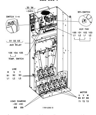
Compact IP 00 without disconnect and fuse VLT 6402-6602 380-460 V and VLT 6502-6652 525-600 V
