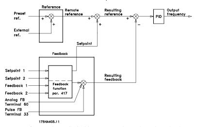
As can be seen, the remote reference is totalled with setpoint 1 or setpoint 2. See also *Reference handling*. Which setpoint is to be totalled with the remote refer-
