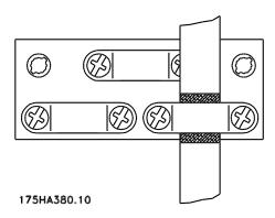
Torque: 0.5-0.6 Nm Screw size: M3
