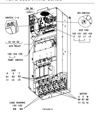
Compact IP 00 with disconnect and fuse VLT 6402-6602 380-460 V and VLT 6502-6652 525-600 V
