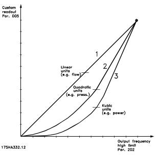
Select a unit to be shown in the display in connection with parameter 005 Max. value of user-defined readout.
