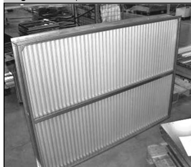
Figure 2b - Drop eliminator
