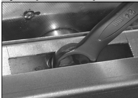
Figure 7 – Tighten the shaft bolt using wrench # 24
