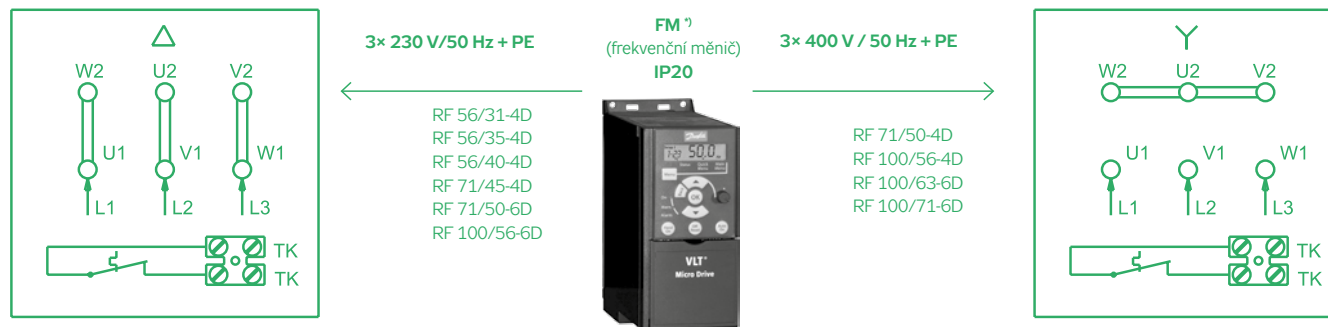
FIGURE 3 – Y/Δ CONNECTION IN THE THREE-PHASE MOTOR TERMINAL BOX WITH FREQUENCY INVERTER, IP 21 (RFFMIMXXXX20)
