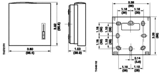
Figure 2. Dimensions in Inches (Millimeters).
