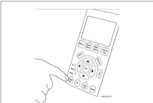
Illustration 4.45: Step 5: By pressing the [Hand on] button, the LED above the button should be lit and the motor may rotate.
