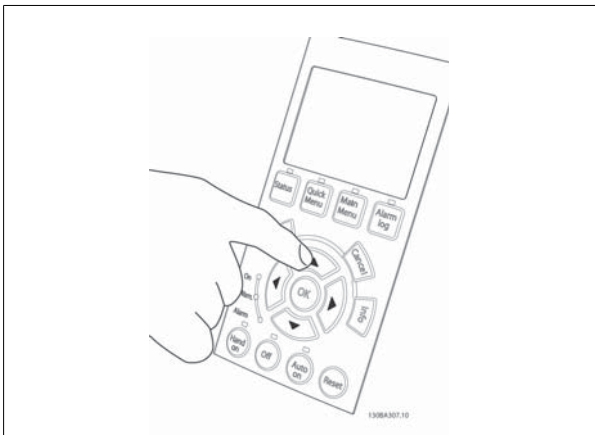
Illustration 4.46: Step 6: The speed of the motor can be seen in the LCP. It can be adjusted by pushing the up ▲ and down ▼ arrow buttons.
