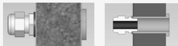
Figure 22 – cable wiring grommet design
